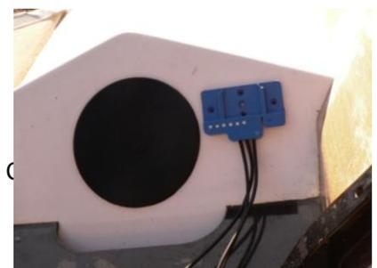
If a heart strap is to be used, then it is important for the HC to be mounted as close as practical to rower. The maximum recommended distance between chest strap and HC is 1150mm.
