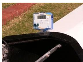
The SRT can be fitted to boat using the blue adjustable bracket or the NK adaptor which fits to the NK cup.
