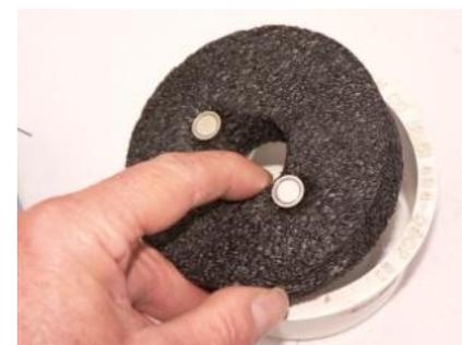
If the NK adaptor is used NK adaptor, then it is pushed into NK cup and SRT attached – via magnets. See pictures on left.
